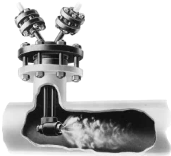
STEAM ATOMIZING DESUPERHEATER
