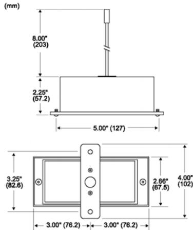
**Figure 1.** Duct Pressure Transducer Dimensions
