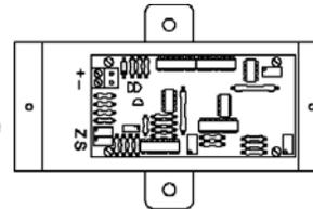
**Figure 3.** Duct Pressure Transducer With mA Output
