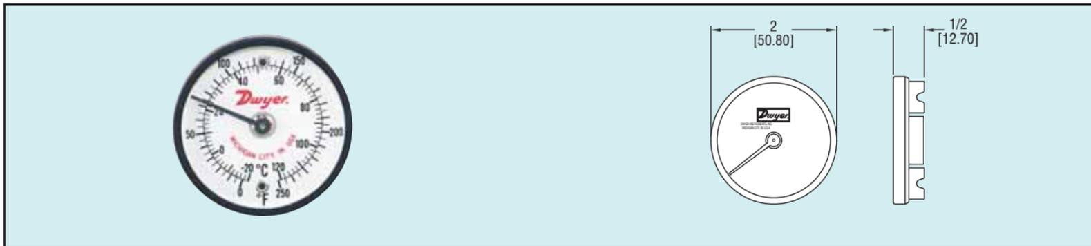
Measure the temperature of boilers, air ducts, motors, bearings, furnaces or other surfaces with Series ST Surface Mount Thermometers. Dual magnet design allows easy mounting on any ferrous surface. Bi-metallic thermal sensing coil provides quick temperature measurement with  $\pm 2\%$  full scale accuracy.
