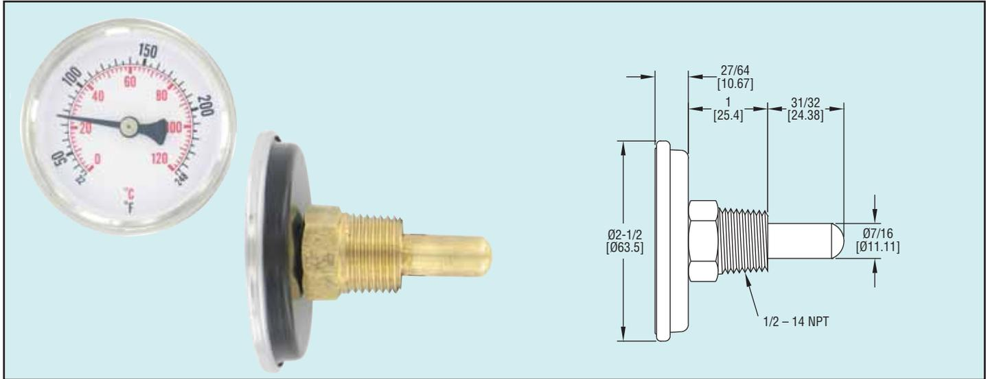
The **HWT250 Bi-Metal Thermometer** is perfect for hot water applications. The dial has dual scales to read in °F and °C. There is an adjustment screw in the stem for easy calibration. Typical applications for the HWT250 would be heating coils, hydronic radiant in-floor systems, and outdoor wood furnaces.
