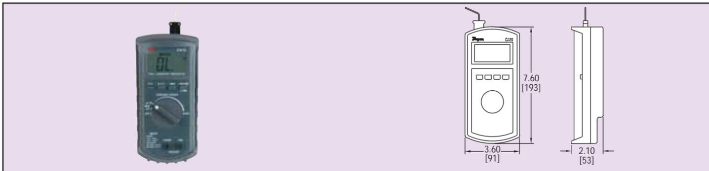
**Dual function CA10 Thermocouple Calibrator** can be used to source Type K thermocouple output values or measure Type K thermocouples. Quickly select output value using the rotary switch with coarse and fine adjustments. Model CA10 accepts up to two Type K thermocouples and features data hold and max functions. Measurements are displayed on a 3-1/2 digit backlit display. Units include a 4" (100 m) Type K bead wire temperature probe, calibration cable, 9V battery and instruction manual.
