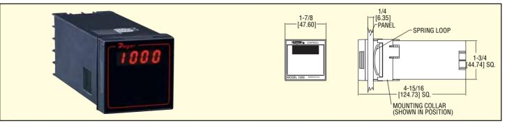
Low cost 1/16 DIN units provide 3-1/2 digit, 0.3" high LED readings from four field selectable input ranges. Includes integral power supply to operate 2-wire transmitters. Optional low/high SPST alarm relays can be set for direct or reverse action.
