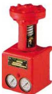
These pilot controllers use an inherently stable force-balanced design and provide high speed response, exceptional reliability and high output volume. Normal operating pressure is 20 to 22 psig, maximum static pressure is 900 psig and the adjustable range is 13 psia to 800 psig.
