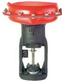
Leslie spring and diaphragm actuators are rugged high thrust units with flanged yoke to bonnet connections for simple maintenance and better access to stem packing. These workhorses of our control valve lines have been proven and perfected for nearly forty years of in-service usage. They are available in four sizes: 35, 55, 85, and 135 in.<sup>2</sup>
