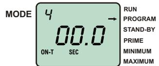
icon will be displayed. The current on time setting will be displayed and the left most (selected) digit will blink. Note: The left most digit can be programmed from 0 - 19. The decimal is fixed and cannot be moved.
