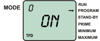
■ Press the DIGIT button to toggle the system on and off.
