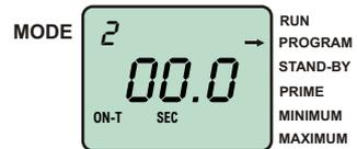
icon will be displayed. The current on time setting will be displayed and the left most (selected) digit will blink. Note: The left most digit can be programmed from 0 - 19. The decimal is fixed and cannot be moved.
