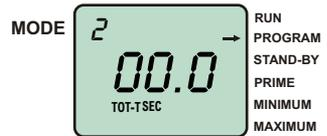
(selected) digit will blink. Note: The left most digit can be programmed from 0 - 19. The decimal is fixed and cannot be moved.
