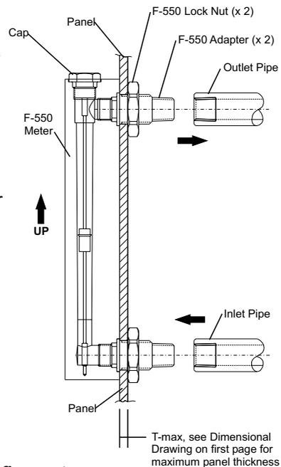
**Cleaning:** The flowmeter body and all other parts can be cleaned by washing in a mild soap and water solution. A soft bristle bottle brush will simplify cleaning inside the meter body. Note the floats up position for re-assembly.
