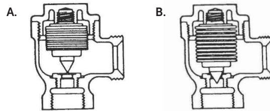
**A.** In a trap which is cold, or which is full of condensate below the boiling point, the Sterlco® thermostat remains compressed because of its internal vacuum. The trap is open and condensate flows out.
