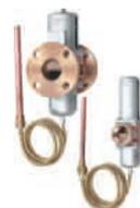
Top Performance. Economical Price. Brass Construction with sizes from 3/8" to 2-1/2" and pressures to 150 PSI. Buna-N seat disc with 6-ft. capillary. 6 standard ranges from 40°F to 275°F.
