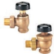
Suitable for 1-pipe steam systems and 2-pipe steam and hot water systems. Pressures to 200 PSI. Models are available with packed, packless and spring packed stems and range in sizes from 1/2" - 2". Body patterns include angle, straightway and corner style.
