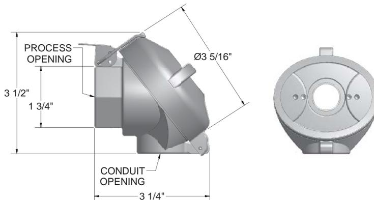
These connection heads are designed for use in hazardous locations; places where flammable or explosive conditions exist. The following connection head types meet CSA or FM standards for hazardous locations and, depending on application, can be used as part of explosion-proof (XP) temperature sensor assemblies in Class I, Division I hazardous locations.
