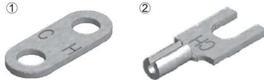
[1] Terminal lugs fit Cinch Jones Series #141 and equivalent Barrier terminal blocks with 27/64" screw spacing and #6-32 terminal screws.
