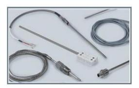
RTD's: Resistance temperature detectors accurately sense process temperatures with an excellent degree of repeatability interchangeability of elements. Also known as resistance thermometers, the RTD is composed of certain metallic elements whose change in resistance is a function of temperature. Pyromation manufactures resistance temperature detectors and resistance thermometers for many industry applications, and has the right RTD type for your job.
