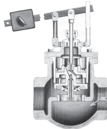
The No. 73 Single Seated Lever Valve is the same as No. 7, shown and described on pages 7 and 8, minus float, float rod and rosette, and plus a counterweight.
