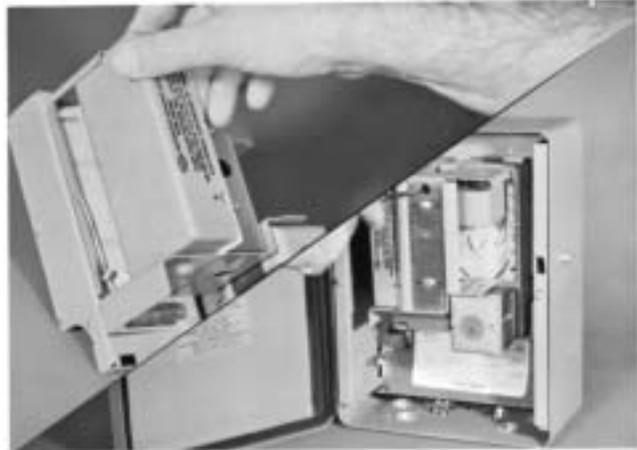
6. Replace the #4-128 Firetron cell in the scanner with the #4-263 firetron cell. Attach the label supplied with the 4-263 Firetron cell to the scanner body.
