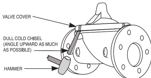
On 6" and smaller valves block and tackle or a power hoist can be used to lift valve cover by inserting proper size eye bolt in place of the center cover plug. On 8" and larger valves there are 4 holes (5/8" – 1 1/2" size) where jacking screws and/or eye bolts may be inserted for lifting purposes. **Pull cover straight up** to keep from damaging the integral seat bearing and stem.
