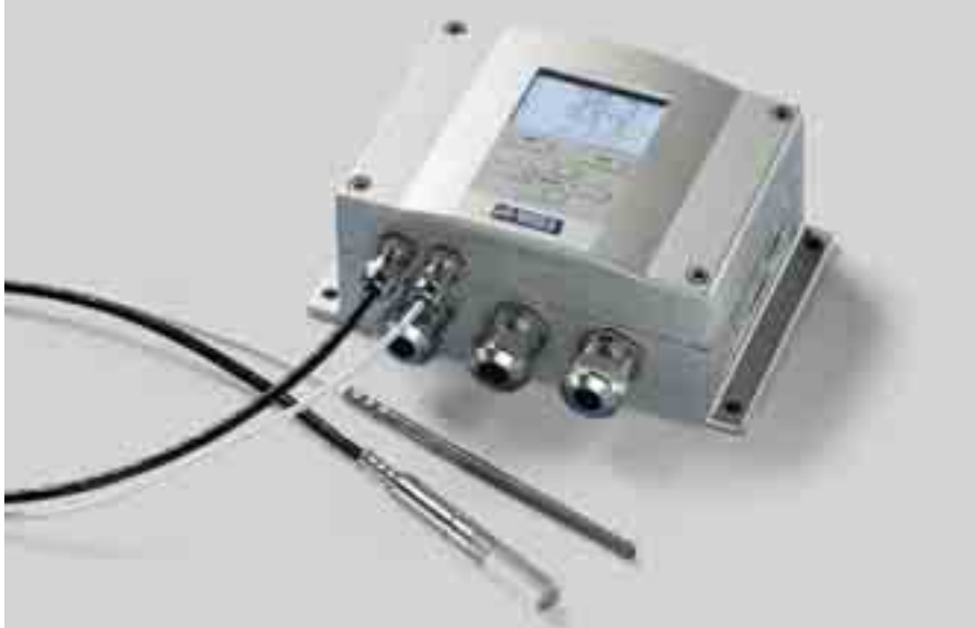
The HMT337 is the ideal transmitter for the most demanding process and meteorological measurements.
