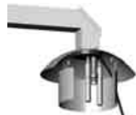
For calibration, a portable HMP77 reference probe is easy to attach beside the HMT337 or PTU307 probe.
