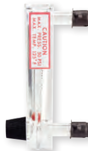
Model MMF mounts easily from front of panel. Drill two 9/32" or 5/16" dia. holes in panel on 2-1/16" centers. Insert mounting connector spuds. From rear, slide on the two spring retainers (furnished) and push on rubber or plastic tubing.
