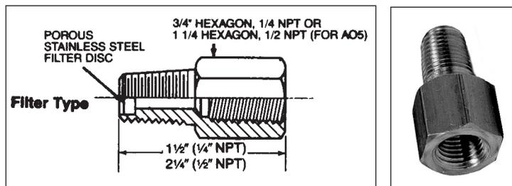
**Filter Type:** Snubbing element consists of a 3/8" diameter x 1/8" thick Micro Metallic stainless steel filter. When placed in the line just before the pressure gauge, the gauge pointer moves across the scale at a rate which is proportional to the pressure differential across the snubber element.
