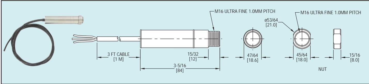
The Series ILA Non-Contact Sensors, measure temperatures from 32 to 932°F (0 to 500°C) and provide a linear 4 to 20 mA, 0 to 50 mV VDC or thermocouple output. The 2-wire signal is compatible with almost any indicator, controller, recorder, data logger, etc., without the need for special interfacing or signal conditioning. They are suitable for most materials such as food, paper, textiles, plastics, leather, tobacco, pharmaceuticals, chemicals, rubber, coal, and asphalt.
