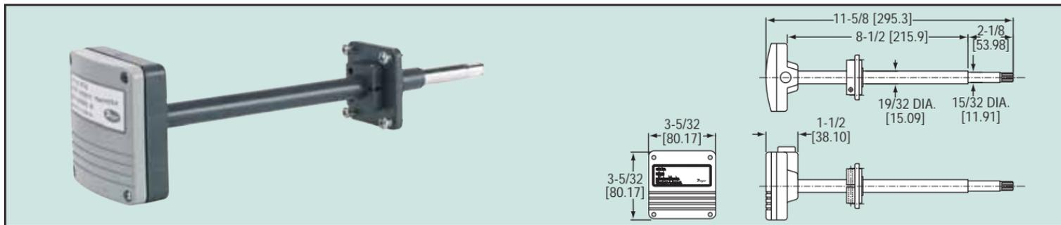
**Monitor and control** relative humidity and temperature in building energy management systems with the Series HT Humidity/Temperature Transmitter. Designed for demanding HVAC/EMCS applications, the Series HT provides  $\pm 3\%$  RH accuracy and  $\pm 1\%$  stability per year. Routine calibration is not required with the fully interchangeable sensor. Two wire connections allow easy installation directly into air ducts or within a controlled area.
