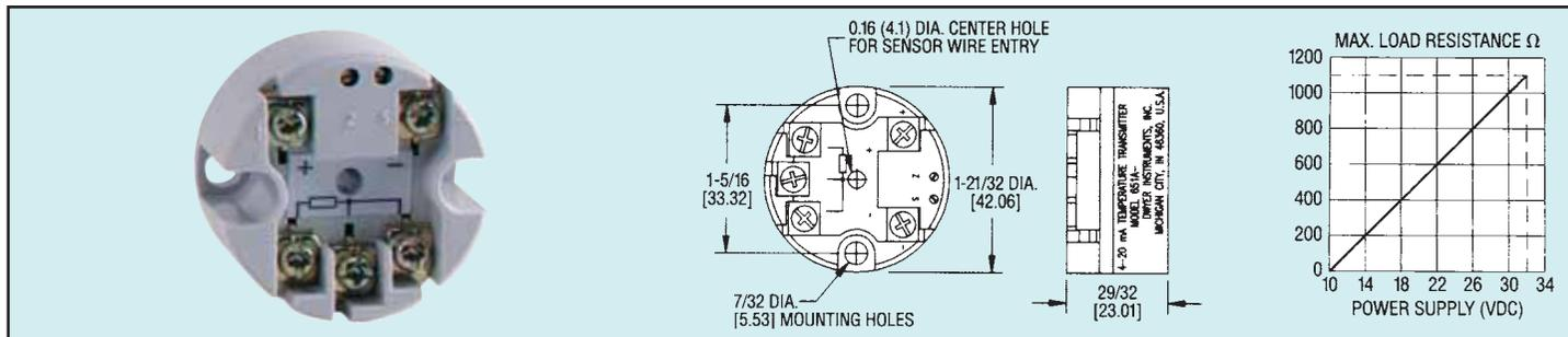
**Linearized output** for precise temperature monitoring or control is combined with small size and quick, easy mounting. Rugged Series 651 transmitters are designed for use with 2 or 3 wire Pt100 RTDs (to DIN standard 43760 or BS1904) or ungrounded Type K thermocouples. Thermocouple models 651TC are cold junction compensated, automatic 32 to 160°F (0 to 70°C) with upscale burnout. These economical devices provide the accuracy and reliability you need at the lowest possible cost.
