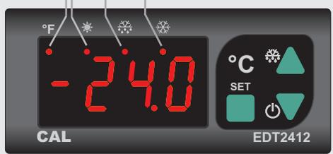
**°F FAHRENHEIT LED:** In parameter value or the measured temperature value "°F" unit while this LED lights up. In the hidden menu at the same time the user menu parameter is shown the LED lights up.
