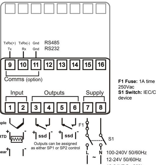
F1 Fuse: 1A time lag type to IEC127. CSA/UL rating 250Vac
