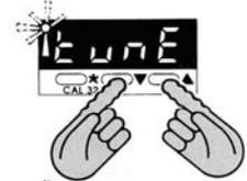
NOTE: Setpoint is locked during **tunE** to adjust
