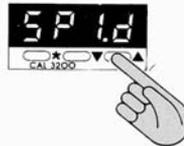
The display shows that no output device has been allocated to SP1
