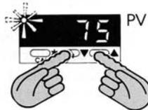
Release together when **tunE** is displayed on entry to program mode. If display differs, **see 2** for functions menu, press ▼ or ▲ to locate **tunE**
