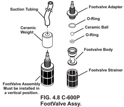
FIG. 4.8 C-600P Foot Valve Assy.
