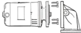
**B)** Remove impeller and screw and motor screws. (Note: opposite end of motor shaft is fitted with screwdriver slot to hold shaft securely while impeller screw is being removed).
