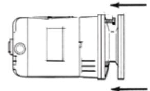
**H)** Lubricate impeller hub with seal lubricant. Slip new bellows and spring onto impeller hub. Be sure bellows slides freely on impeller hub.
