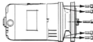
**C)** Insert two of the pump screws into the two threaded holes in the bracket. Tighten them slowly and evenly to force the impeller and bracket off the shaft. Do not pry the impeller or bracket!
