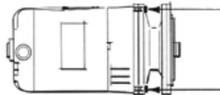
**D)** Remove old seal parts from impeller hub and bracket. Be sure water slinger is in place.
