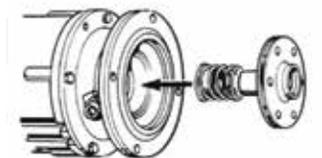
**I)** Replace impeller on motor shaft and secure with impeller screw. Hold shaft with screwdriver slot while tightening screw.
