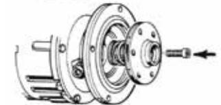
**J)** Replace pump housing onto bracket, using a new housing gasket. Secure with pump screws. Be certain gasket is seated properly.
