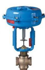
Flowrite II Heavy Duty Bronze Globe Control Valves. Flowrite II 593 Series Utility bronze control valves for steam/water modulation, mixing or by-pass applications. Safety features protect your process and your personnel. Balanced and unbalanced designs. Multiple packing choices - spring loaded. Stainless steel hardware and actuator mounting accessories. Available with pneumatic diaphragm. Union and screwed ends. Multi-guided stability.
