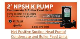
The <u>Sterlco<sup>®</sup> K Series 2' NPSH</u> Pump is designed to pump hot condensate up to 212° F on elevated tank units. If a steam trap fails in the system, this unit will continue to operate up to 12° higher than standard units. The added inducer increases vapor pressure and prevents the whole system failing from pump cavitation.
