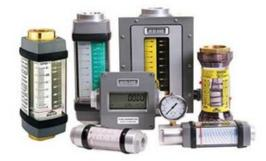
Variable Area Flow Meters: The Hedland product line features over 15,000 inline, variable area flow meters to measure oil, phosphate esters, water, water-based fluids, pressurized air and other compressed gases. Hedland products work well for both new and retrofit applications as they can be installed in any position, do not require flow straighteners, and have no special piping requirements.
