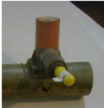
ALDYL-A TEE AFTER SCRAPING
