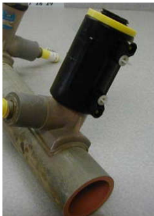
A COMPLETED ELECTROFUSION OF ALDYLA TAP TEE USING KEROTEST REPAIR KIT P/N 72770515
