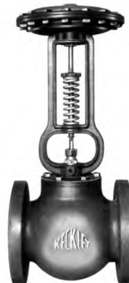
On self contained regulators for reduced pressures above 60 psi, a piston operator is necessary and replaces the diaphragm operator at additional cost.
