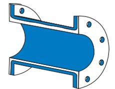
Pinch Valve Double Wall Sleeve
