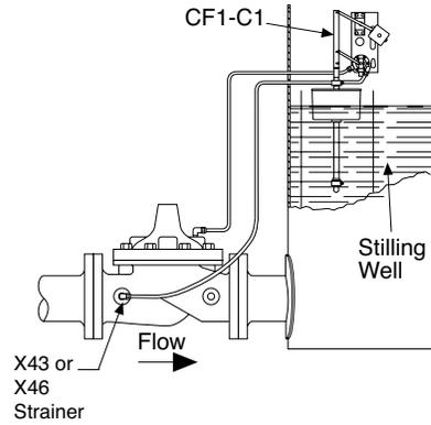
Note: We recommend protecting Float Control tubing and valve from freezing temperatures.
