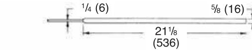
STYLE NO. 712 —Plain Bulb with 1/4" OD Bendable Tubing Cover for Capillary. Used in open tanks or where a mounting connection is not required.
