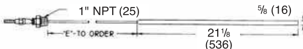
STYLE NO. 731 —Plain Bulb with Adjustable Extension. Used in oil storage tanks or wherever it is desirable to change position of bulb. Dimension "E" must be specified.
