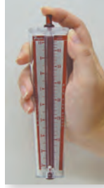
For high scale reading, finger covers hole
