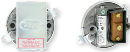
Series 1910 switch with conduit enclosure off. Shows electric switch and set point adjustment screw located on same side for easy installation.
