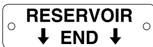
This brass plate appears on altitude valves only and is found on top of the outlet flange.
