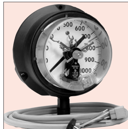
Indicating accuracy of Royal Gauge, above 300 psi with contact: Pointer not carrying contact – 1.0%. Pointer carrying contact – 1.5%. For ranges below 30 psi, add an additional ½% to indicating accuracies.
