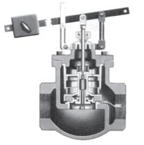
The No. 73 Single Seated Lever Valve is the same as No. 7, shown and described on pages 7 and 8, minus float, float rod and rosette, and plus a counterweight.
