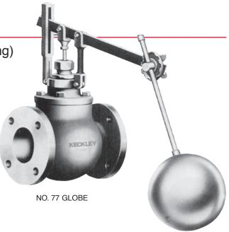
Application/Service: The No. 7 and 77 pilot controlled float valves are recommended when tight closing is essential. They are commonly used to maintain a water level in an open tank. They are best suited for clean liquids not injurious to neoprene, leather or brass parts. Standard design temperature is 125°F. For higher temperatures up to 350°F, the neoprene disc in the No. 7 or neoprene disc and leather cup in the No. 77 are replaced by teflon parts.
