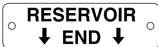
This brass plate appears on altitude valves only and is found on top of the outlet flange.
